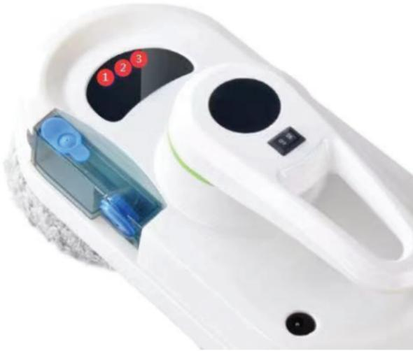
**The first light (1)**, to the left, signals the state of the battery. When the battery is low, incomplete, or charging, the light will turn red. When the robot is fully charged, the light will turn blue.
